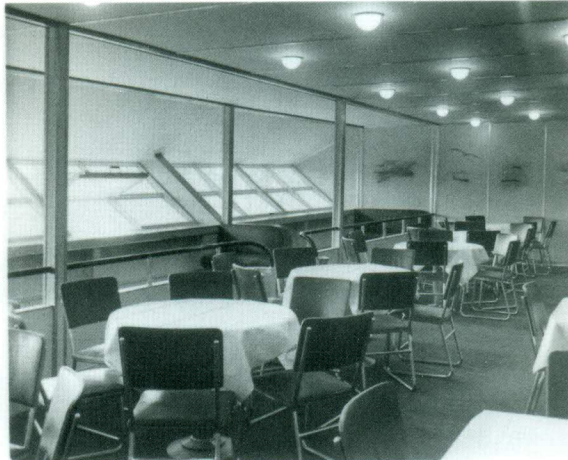
View 23 from a German series, "Hindenburg, Speiseshal." (Dining room on the Hindenburg.) A view looking from the dining room, across the promenade area to the angled windows that provided excellent views of the ground below. While the passenger rooms were compact, the dining room and promenade were quite spacious for an airship. The tables and chairs were specially made for the Hindenburg, and were very lightweight.
