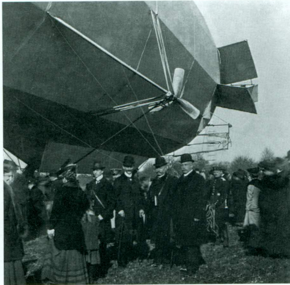
Enlarged detail of an NPG view of LZ-3 showing details of the rear portion of the airship. Note the long drive shaft that connected the propeller to the engine in the open gondola, and the bracing of the propeller assembly to the airframe. Also note the angled stabilizing fins at the rear with rudder panels between them, and the four level elevator fins at the bottom of the tail of the zeppelin. (Courtesy Martin Kohler)
