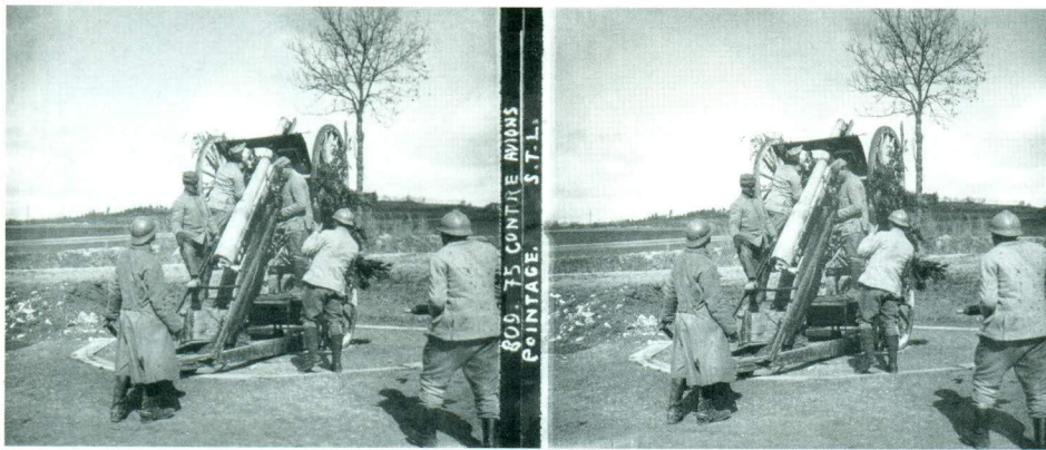
An Editions STL glass view of a makeshift anti-aircraft gun. Before the development of specially designed anti-aircraft guns, field guns were put on a variety of makeshift mounts to convert them into anti-aircraft guns. Here a French 75mm field gun has been set to fire at a high angle on a rotating gun mount. The addition of tree branches on each side of the gun is a curious form of camouflage in such an barren and exposed position. Later, the German Flak 102, an 88mm anti-aircraft gun was developed in 1917. It had a rate of fire of 10 rounds a minute, and a range of 12, 600 feet vertical, and 11,800 yards horizontal.
