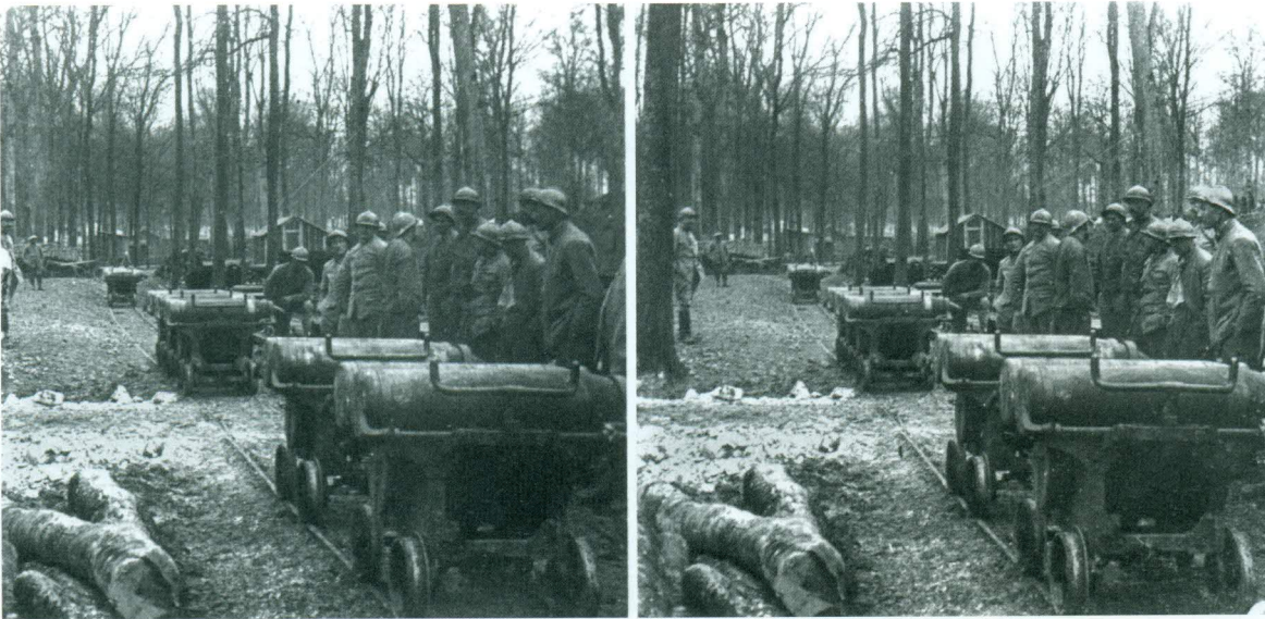
..... "Somme-transport l'obus" (Transport of shells on the Somme). This is a French glass view from the Brentano's Over There set sold in the USA after the war in Brentano's book stores. Shells for a heavy gun are transported from the supply depot to the gun by a light gauge rail line on hand carts that hold two shells. Light gauge railways such as this were used to move men, ammunition, and supplies from the supply depot to the front lines. .....
