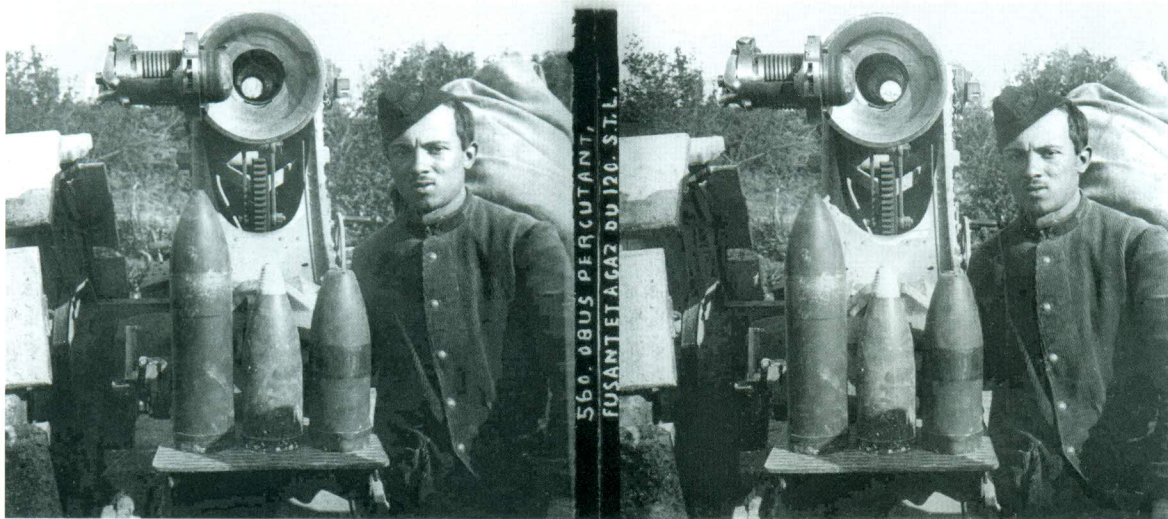
"Obus percutant, fusant et a gaz du 120" (120 Shells for hitting, fusing and gas). A French glass view by Editions S.T.L. of the Model 1878, 120mm, 5", field gun. The three main types of shells for artillery in WW1 are on display, as well as the open breach of the gun. The shell on the left is a high explosive shell, designed to burst on impact or with a short delay, to let the shell burry itself and do more damage. The shell in the center has a timed fuse on the nose, and it is probably a shrapnel shell, which
