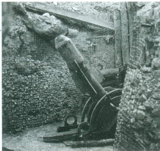
"Un crapouillot et sa torpille." (A Toad and a torpedo.) The French called this style of trench mortar a Crapaud, or Toad, for the way they hopped in recoil. A rod was welded to the base of the mortar bomb and fit down into the barrel of the mortar. The fins insured that the bomb landed nose first. Trench mortars were greatly feared and respected by both sides, as they delivered a very large amount of explosive. The nature of trench war created the need for the infantry to have their own artillery close at hand, and trench mortars and infantry guns were developed. (Collection of Robert Boyd)
